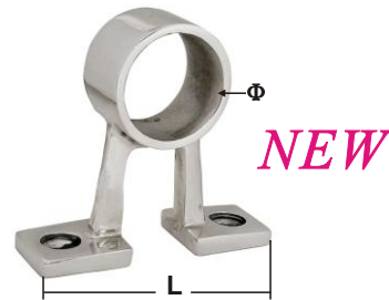
HANDRAIL CENTER FITTING/ PASSAGE MAIN COURANTE casted AISI 316 ITEM NO. \Phi mm L mm Weight/g B23-005 25 65 90
