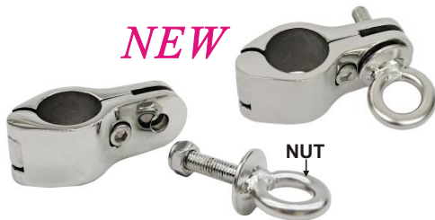
TOP SLIDE WITH NUT casted AISI 316 Ideal for installing bimini tops stringers for fender racks or wherever a rail mounted hinge is commonly needed ITEM NO. Tube O.D. B23-002 22mm(7/8") B23-003 25mm(1")
