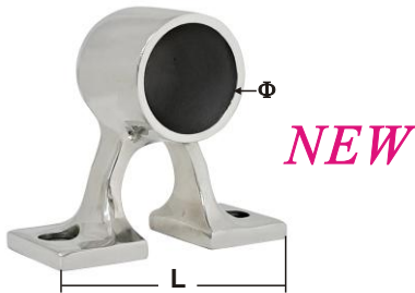
HANDRAIL END FITTING/ EMBOUT MAIN COURANTE casted AISI 316 ITEM NO. \Phi mm L mm Weight/g B23-004 25 65 160
